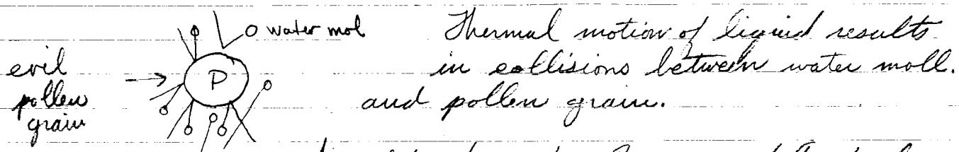
Simplify to 1-d. Because of Central Limit Theorem, motion should follow normal dist. Moreover, the var grows linearly w/ time, because of lack of memory.
